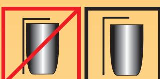
A gap between crucible and a furnace cover should be insulated by thermoinsulating material.
