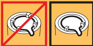
Around of an upper crucible edge it is necessary to create an equal gap. For this purpose it is possible to use cardboard or arboreal chips. It is not allowed to use wedges made of fire proof material.
