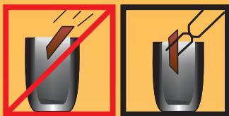
The metal is loaded only into a heated crucible.
