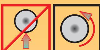
The burner should be installed so that the flame does not beat directly into the crucible, but bends around it tangentially.
