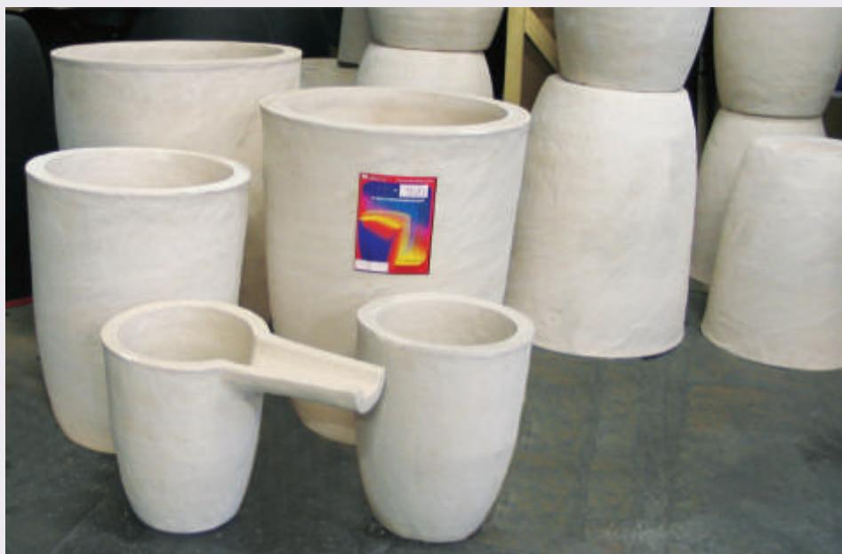
The plant accepts orders for the manufacture of crucibles with dimensions not listed in these tables
