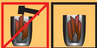
The ingots should be laid into a crucible vertically
