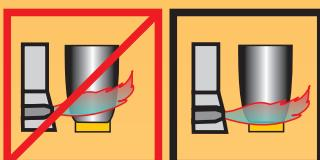
The burner axis should be in a bottom plane of a crucible.
