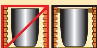
The space between crucible and inductor is filled by insulating material in induction furnaces.
