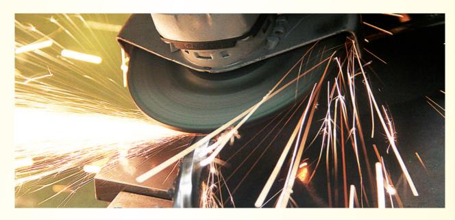
Wheels can be used on angle grinders with number of rotations not exceeling indicated on the wheel value
