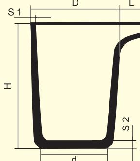
● **Crucibles type ZPX** are glazed cylinder crucibles with a nose for metal tapping intended for operations in the rotating furnaces with the melting temperature up to 1500°C
