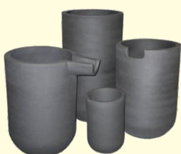
● **Crucibles type ZX** are glazed cylinder crucibles intended for melting of non-ferrous metals and alloys with the melting temperature up to 1500°C in the high-frequency furnaces (10 000-60 000 Hz)
